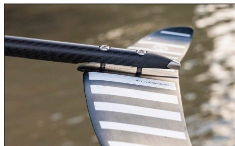
9. Using the 20mm dome head M6 T30 screws, attach the stabiliser to the fuselage.
