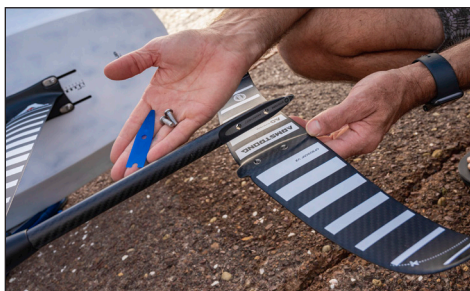
8. Putting the board on its side makes it easier to mount the stabiliser components.
