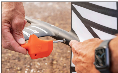
7a. Turn the foil on its side to install the front foil barrel nut.
